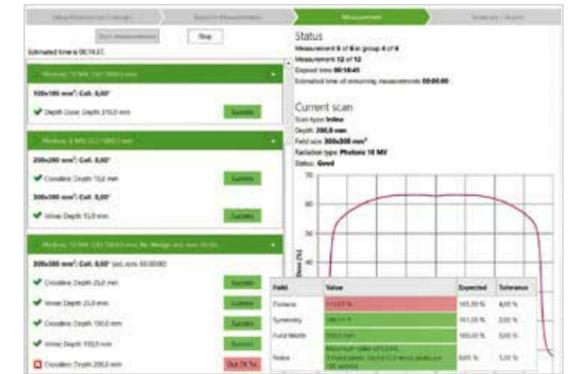
Automatic scanning with instant check of each scan for flatness, beam symmetry, leakage and signal noise. Immediate warnings in case of suspicious scans.
