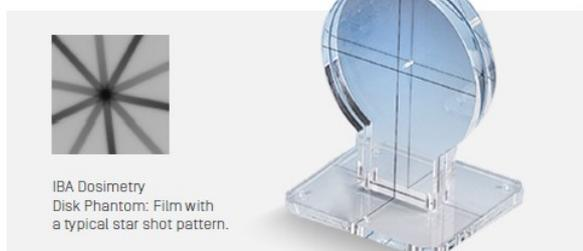
For determination of the isocentric accuracy. The film is held between the two perspex disks and a tool provided defines the center of crosshairs on the film.
