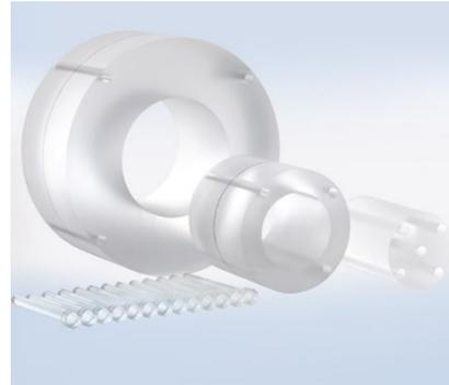
Adult Head & Body / Pediatric Head & Body Innovative 3-part nested PMMA phantom for CTDI measurements. Designed to image pediatric and adult head and body in accordance with FDA performance standard for diagnostic X-ray systems (21CFR 1020.33).
