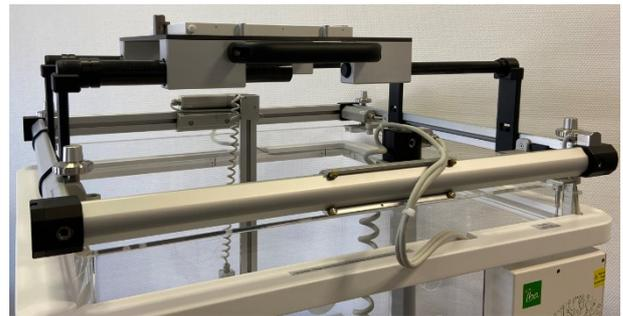
Stealth reference chamber including special holder for Varian® Halcyon™ / Ethos™ (\*) – Linac allows field-size measurements up to max. 28x28 cm without excursions into Linac room for reference chamber re-alignment.
