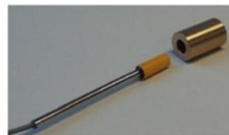
A PFD 3G-pSi diodes and a brass build-up cap
