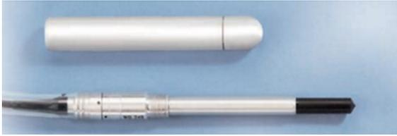
The Farmer type chamber FC65-P is an air cavity ionization chamber, vented through a waterproof silicon sleeve. It is waterproof and fully guarded.
