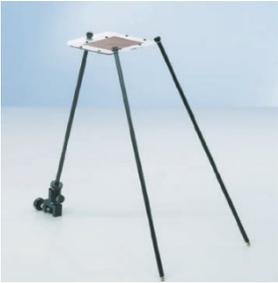
Detector holders for cylindrical and parallel plate chambers:
