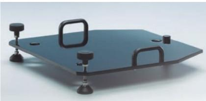
WP1D SCU version, equipped with lead filter for photon beam quality determination and leveling plate:
