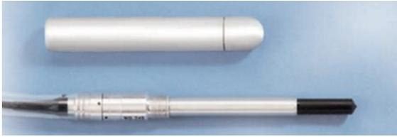
FC65-G ionization chamber for reference dosimetry and calibrations.
