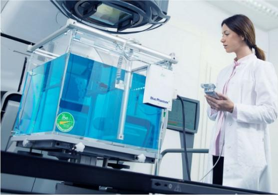
3D Water Phantom System **Blue Phantom<sup>2</sup>** for complete Linac Commissioning & QA
