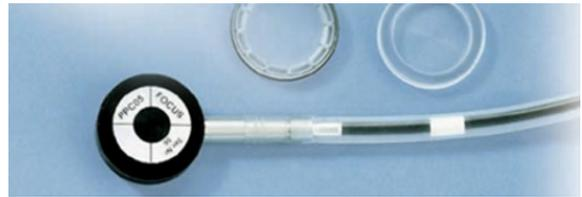
The parallel plate ionization chamber PPC05 is designed for **absolute and relative electron beam dosimetry** above 2 MeV in the measuring quantity absorbed dose to water.
