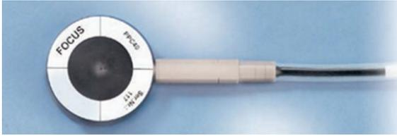
The parallel plate ionization chamber PPC40 is designed for absolute and relative electron beam dosimetry above 2 MeV in the measuring quantity absorbed dose to water.
