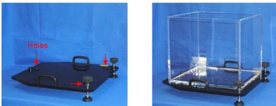
Leveling plate and WP1D -Tank on leveling plate
