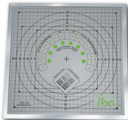
The IBA Dosimetry Primus A test phantom for automated 2D kV image QA with myQA Machines. More information on page 16
