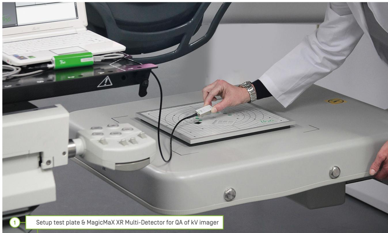
1 Setup test plate & MagicMaX XR Multi-Detector for QA of kV imager
